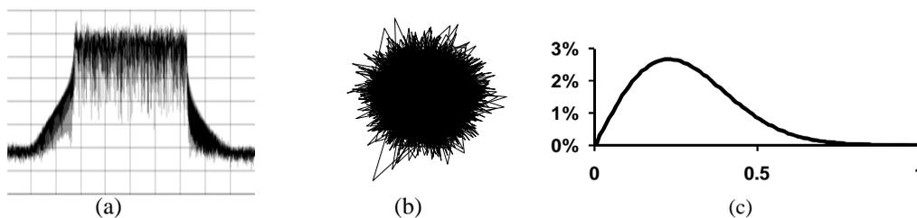
Fig. 9. Representative OFDM signal characteristics: a) measured WiMAX signal power spectral density, b) a simulated vector diagram showing the “peaky” envelope characteristic, and c) its Rayleigh shaped PDF diagram
