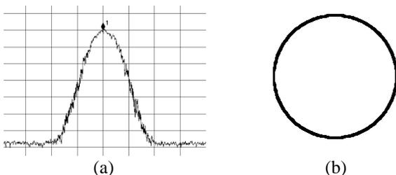
Fig. 1. The NBFM signal: a) one representative power spectral density, and b) its vector diagram showing the constant envelope property.
