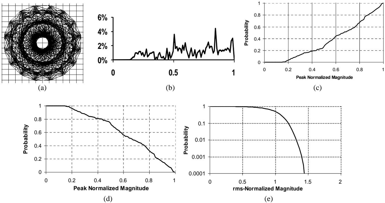
Fig. 2. Examples of envelope statistic measures: a) the example signal vector diagram, and the corresponding curves for b) the PDF, c) the CDF, and d) the CCDF; e) It is more common to normalize the CCDF curve to rms signal power and to show the probabilities on a logarithmic scale.
