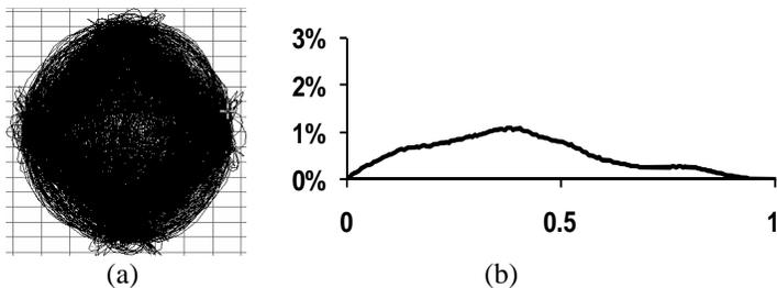
Fig. 7. Representative HSPA signal characteristics: a) a vector diagram, and b) a PDF curve
