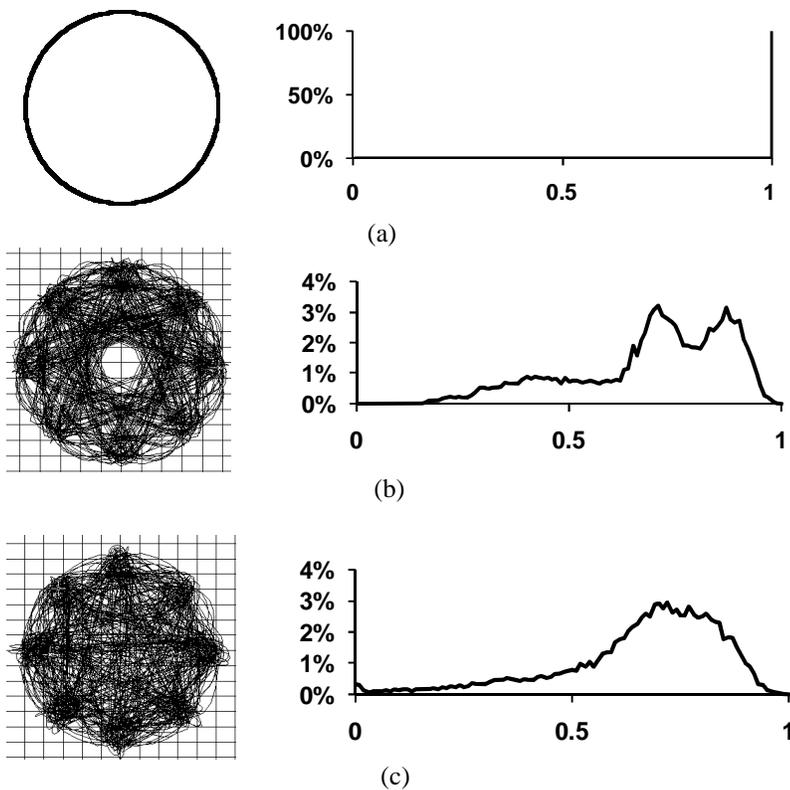
Fig. 8. Bluetooth signal characteristics evolution: vector diagram and envelope PDF curve for a) original Standard, b) EDR, and c) EDR 2.1
