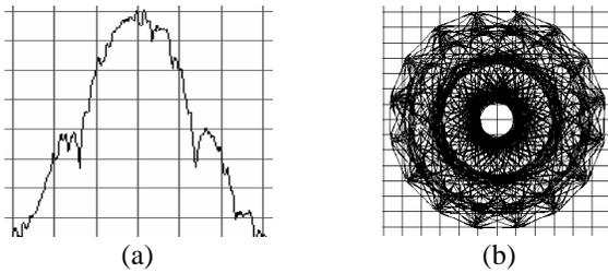
Fig. 5. The EDGE 8PSK signal: a) power spectral density, and b) vector diagram showing envelope varying characteristics
