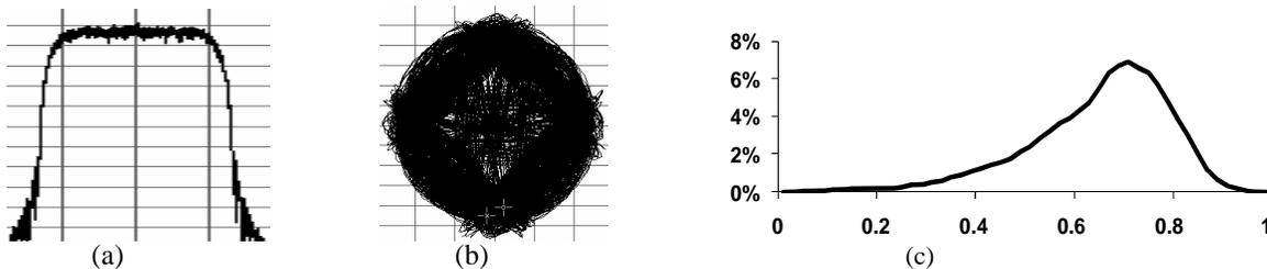
Fig. 6. The UMTS signal: a) power spectral density, b) one representative vector diagram showing envelope varying characteristics, and c) a PDF curve
