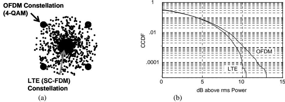
Fig. 9. The LTE signal: a) constellation diagram compared to OFDM for identical information, and b) comparing LTE CCDF characteristics with OFDM
