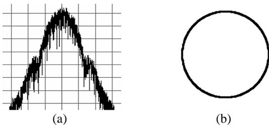
Fig. 4. The GSM GMSK signal: a) power spectral density, and b) vector diagram showing the constant envelope property.
