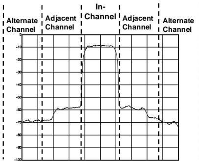
Fig. 3. Definitions of adjacent channel power and alternate channel power
